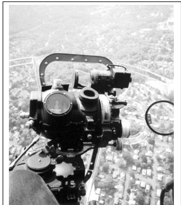
The Norden bomb sight, focused on Latham. It was used to determine the target to be bombed. The navigator/engineer is looking through the sight to get a fix on their location.
