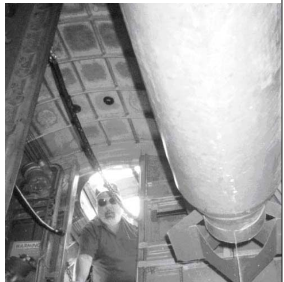
Ron looking into the aisle or bomb bay with the bomb in the foreground. When the bottom bomb was released, all the bombs in the rack followed.
